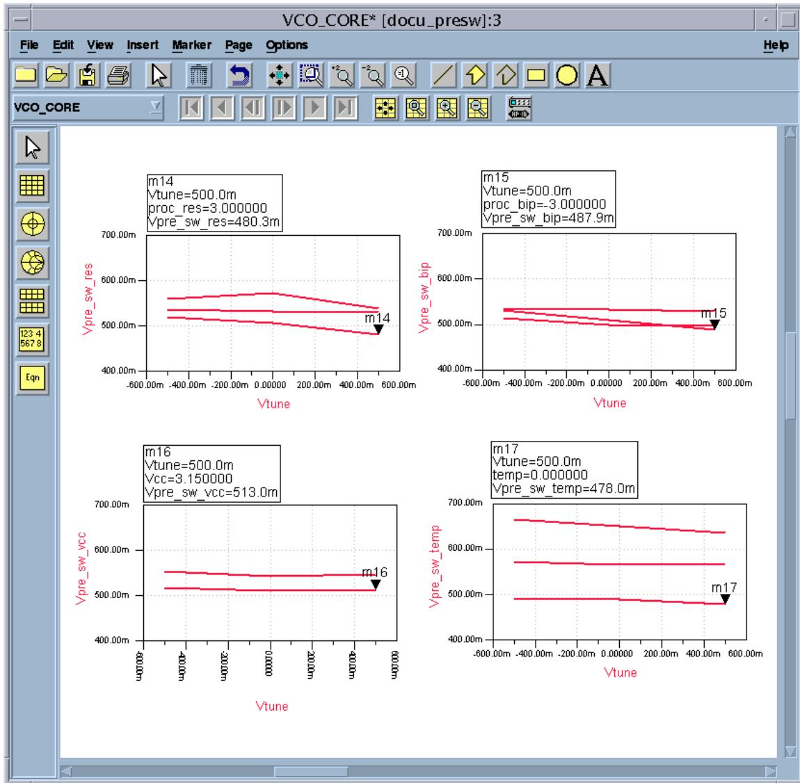
The voltage amplitudes (differential, Vpp) at the output of External Buffer, under variations of process/supply/temperature are shown. The amplitude is  $>600\text{mVpp}$  differentially, enough to drive external  $50\Omega$  transmission line and test instrument for testing. The high amplitude is also sufficient to drive PD, which is in another package, if needed.
