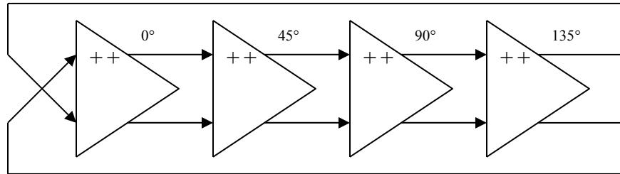
The overall delay through the loop will determine the oscillation frequency (Fosc). If the delay per stage is Td, then the Period of oscillation is  $8 \cdot Td$  and  $Fosc = 1/(8 \cdot Td)$ .
