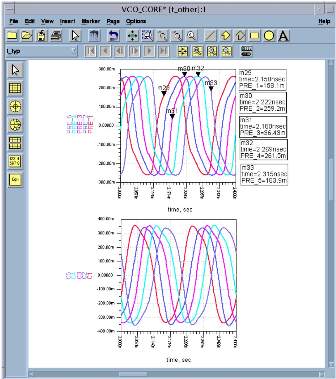
Harmonic Balance is run and the results for a typical operating condition are shown. AP & AN is the waveform at the VCO Core whereas ISO\_AP & ISO\_AN is the waveform at the Isolation Buffer. Their differential waveforms are also shown. Their 3<sup>rd</sup> harmonic are -31dBc and -11dBc respectively.
