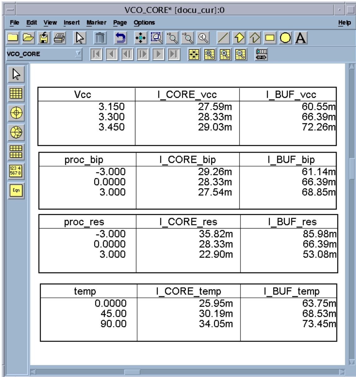
The screenshot shows a software application window titled "VCO\_CORE\* [docu\_cur]:0". The window contains four tables of data, each with three columns: "Vcc", "I\_CORE\_xx", and "I\_BUF\_xx". The tables are arranged vertically. The first table is for Vcc, the second for proc\_bip, the third for proc\_res, and the fourth for temp.
